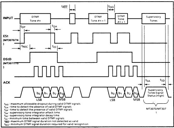
Figure 2 - Timing Diagram
