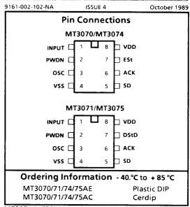
MT3071/MT3075 uses internal counters to provide a preset DTMF validation period. The MT3070/MT3071/MT3074/MT3075 uses a crystal or a ceramic resonator to complete the oscillator circuit.
